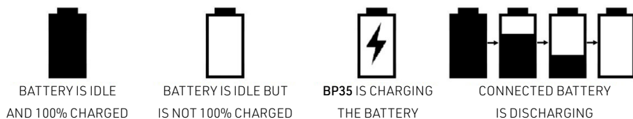
Figure 4: RVView2 battery status indications
